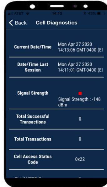
Unsuccessful: Additional field are shown. Cell Access Status Code contains an error.
