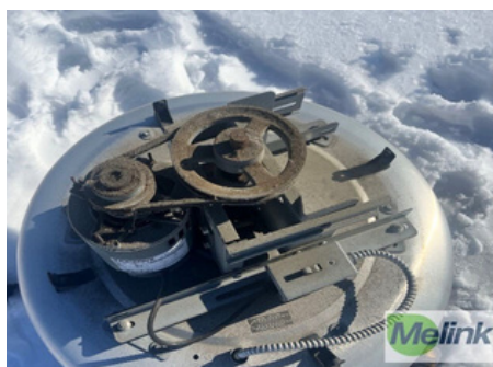
Exhaust fan without a working motor when switched on and breaker set to on.
