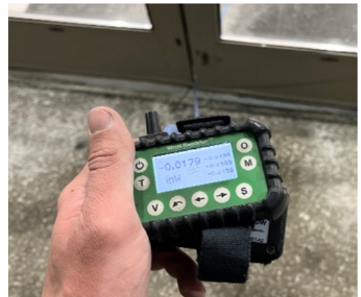
Negative building pressure when overall pressure should be positive.
