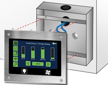
Attach the Touchpad to the Surface Mount box using the four 6-32 machine screws.
