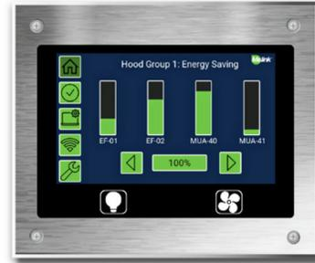
Set the Touchpad address through the Configuration Menu. See Operations manual for details. Each Touchpad must have a unique address.
