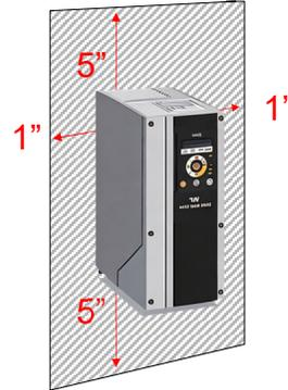
The location must be relatively free of dirt, grease, and water. The ambient temperature must be between +14 degrees F and +122 degrees F. There should be 5" of clearance on the top and bottom and 1" on the sides for adequate ventilation/cooling.
